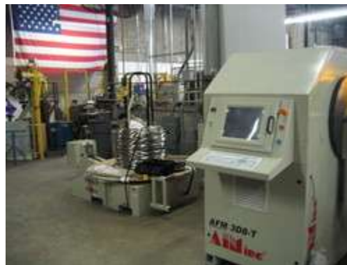
Fastest CNC Wire Form Robot-495 inches of wire per minute bending at a rate of 3600 degrees a second.
